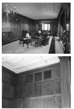
FIGURES 11-12 Linear diffusers located in the plaster walls at each end of this 1917 executive suite increase air supply volume and coverage. reducing the number of wall penetrations otherwise required for conventional grilles. Louvered grilles were confined to end bays and grain painted to blend with the room's paneled oak walls.
