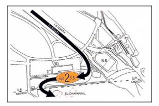
Option 2: East-West Alignment of the Southbound Inspection facility with expanded Northbound Primary Inspection Lanes
